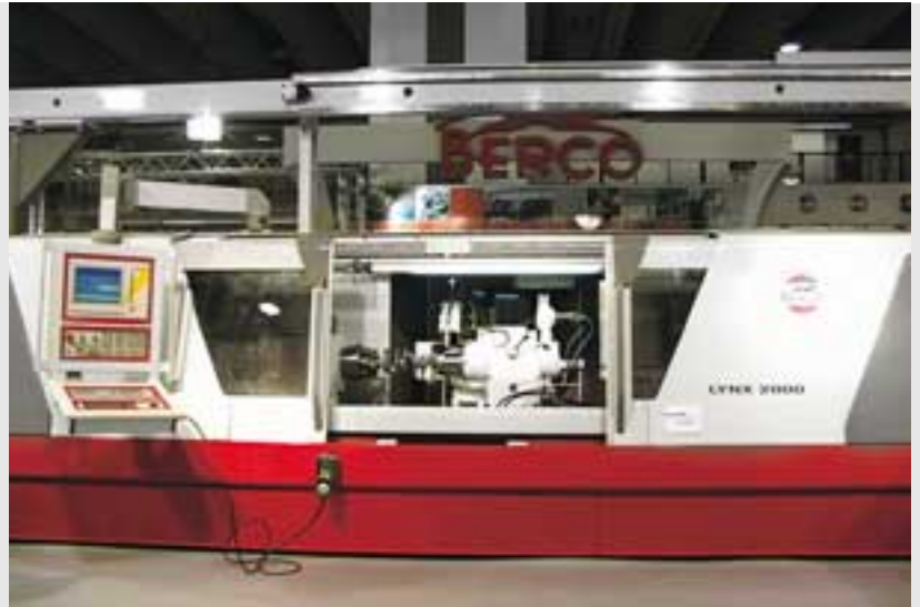
General view of the LYNX 2000 orbital grinding machine from Berco SpA for maximum precision shaft machining.
