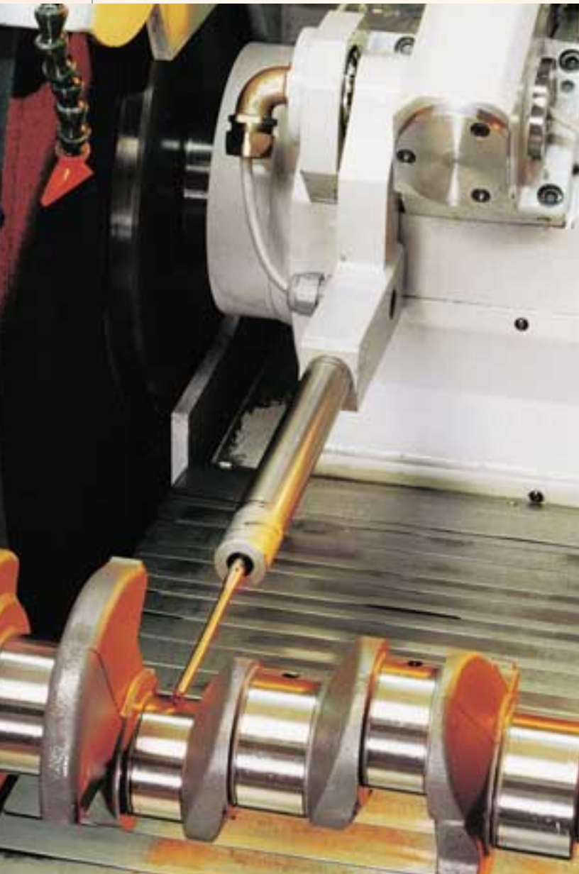
Mechanical probe during measurement of the crankshaft.
